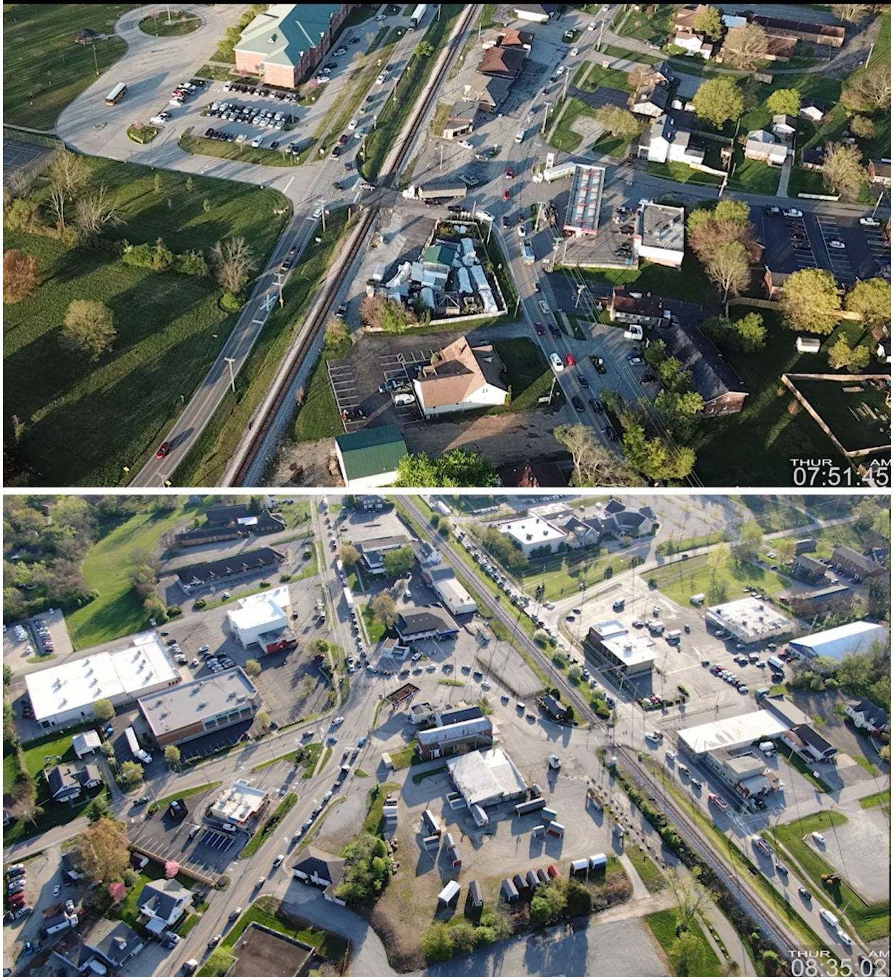
Figure 3: AM Queue Lengths during I-71 Lane Closure
